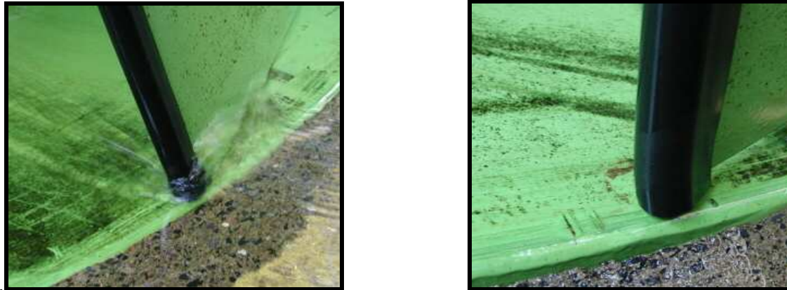
Figure 12. Modified leading edge with rubber extrusions
